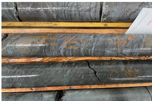
Nickel, copper, cobalt and zinc can be seen with the naked eye in the Surimeau drill core.
