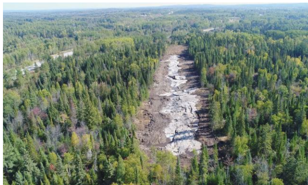
Discovery Vein stripping was carried out on 270m of the known 500m length.
