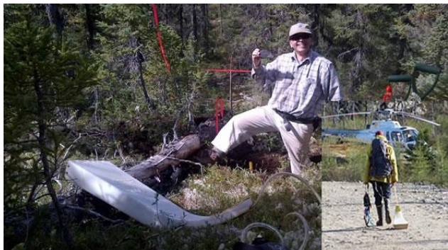
A Beep Mat is used to conduct an efficient, user-friendly, inexpensive electromagnetic survey.
