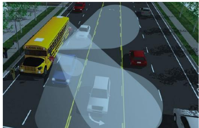
Gatekeeper's technology is able to capture license plates of vehicles in lanes 2, 3, and 4 with high, with its latest 10 megapixel stop arm camera system.
