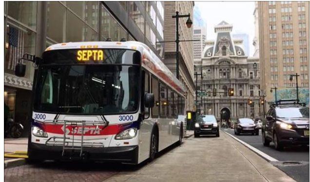
SEPTA's New Flyer Xcelsior XDE40 bus in Philadelphia. This bus is equipped with a Cummins ISL, an Allison EP40 HybriDriv, and soon a Gatekeeper high definition multi camera system.
