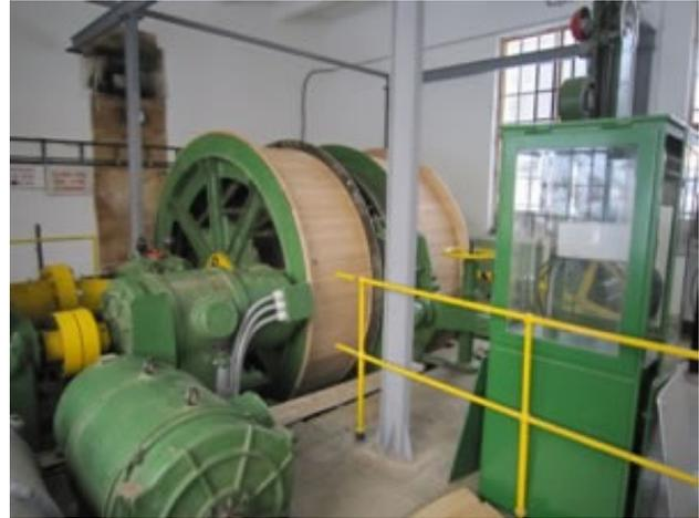
**The hoisting mechanism at Strieborná to get people and equipment up and down the 250 meter deep shaft has been fully restored.**
