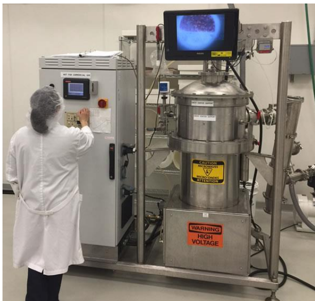
A lab-scale freezeREV unit designed to provide high-speed dehydration for live and active organisms in vials.
