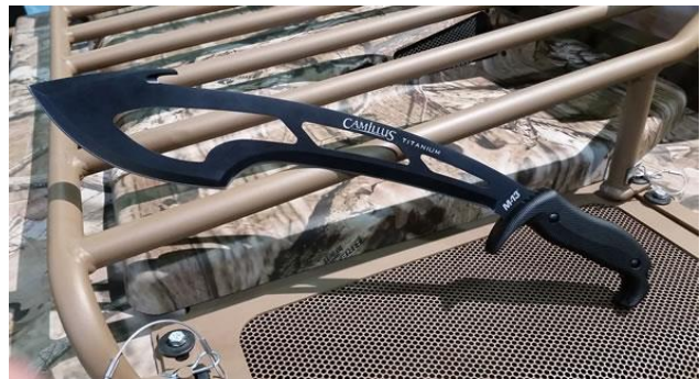
The Camillus M-13 Machete, featuring a 13" titanium bonded blade with gut hook.
