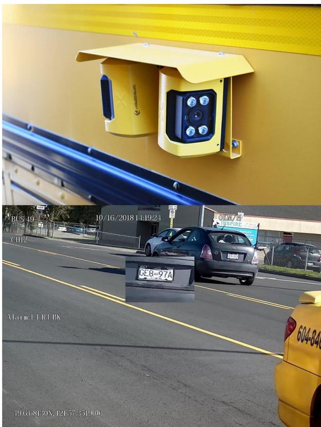
**Gatekeeper's technology is able to capture license plates of vehicles in lanes 2, 3, and 4 with high, with its latest 10 megapixel stop arm camera system.**
