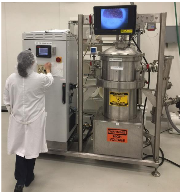
A lab-scale freezeREV designed to provide high-speed dehydration for live and active organisms in vials.
